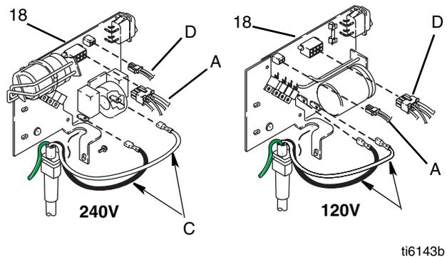
5. Connect motor connector (D) and pressure control assembly connector (A).
