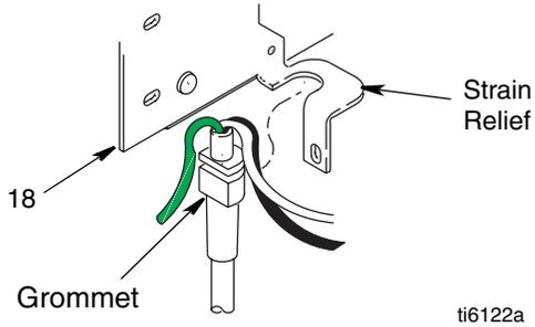
2. Connect power cord connectors to terminals indicated on control board (18).
