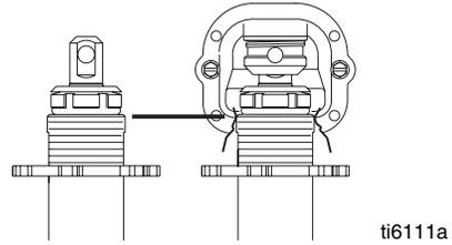
6. Align pump outlet (E) to back.
