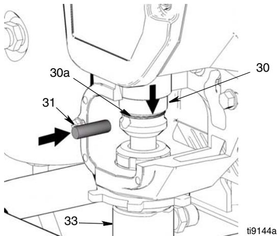
4. Push pump (33) up until pump threads engage.
