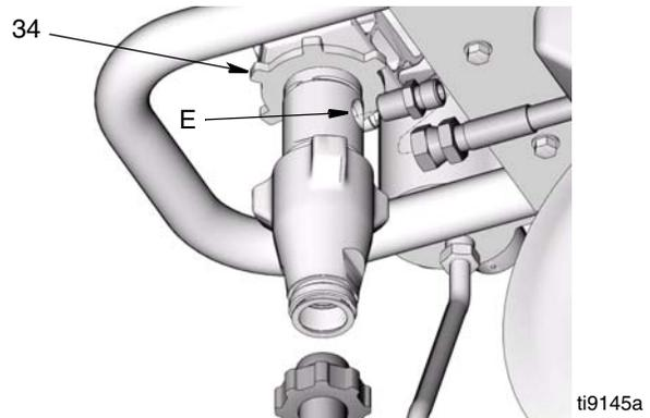
7. Screw jam nut (34) up onto pump until nut stops. Tighten jam nut by hand, then tap 1/8 to 1/4 turn with a 20 oz (maximum) hammer to approximately 75 ft-lb (102 N•m).
