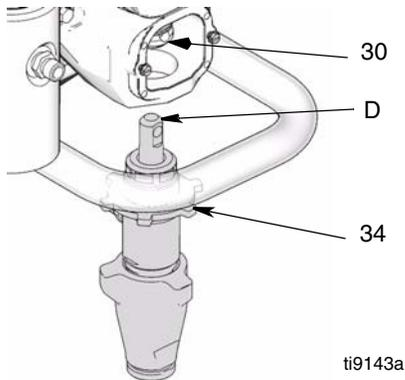
2. Install pump rod (D) into connecting rod (30).
