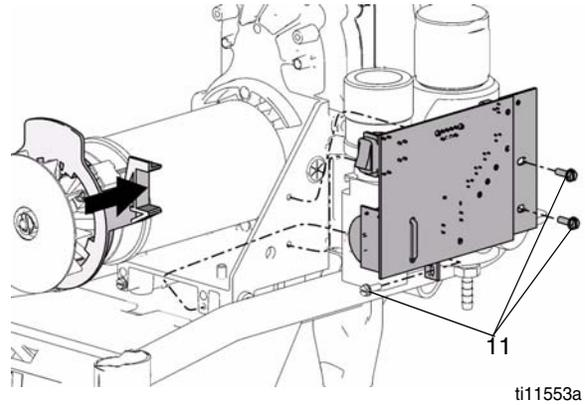
4. Replace three screws (11). Torque to 30-35 in-lb (3.4-3.9 N.m).
