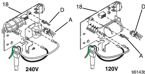
5. Disconnect motor connector (D) from control board (18).
