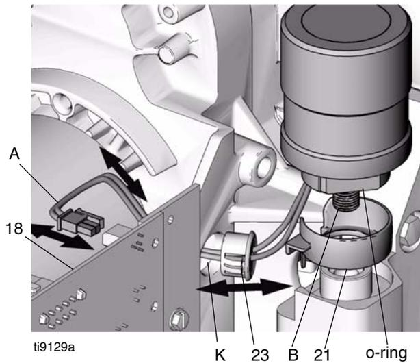
1. Inspect pressure control before installation to verify o-ring is installed.
